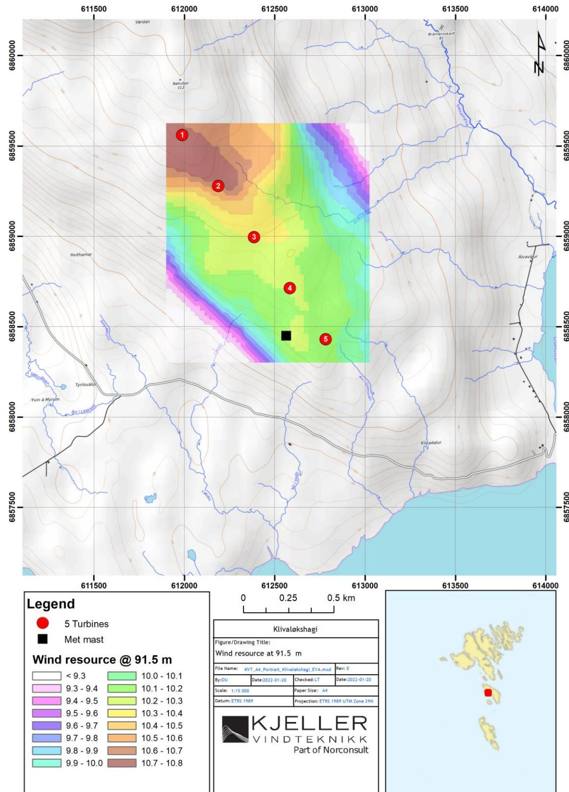
Figure 7. Wind resource map valid at 91.5 m AGL at Klivaløkshagi (together with 5 turbine layout).
