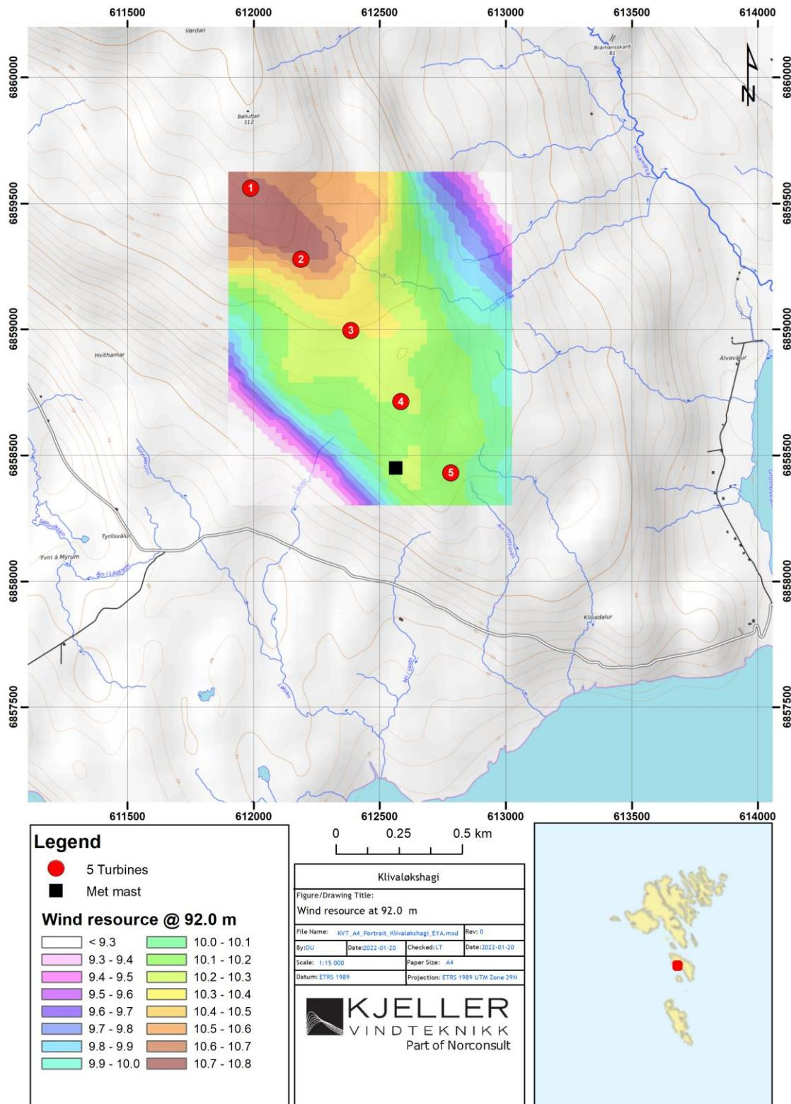
Figure 8. Wind resource map valid at 92 m AGL at Klivaløkshagi (together with 5 turbine layout).
