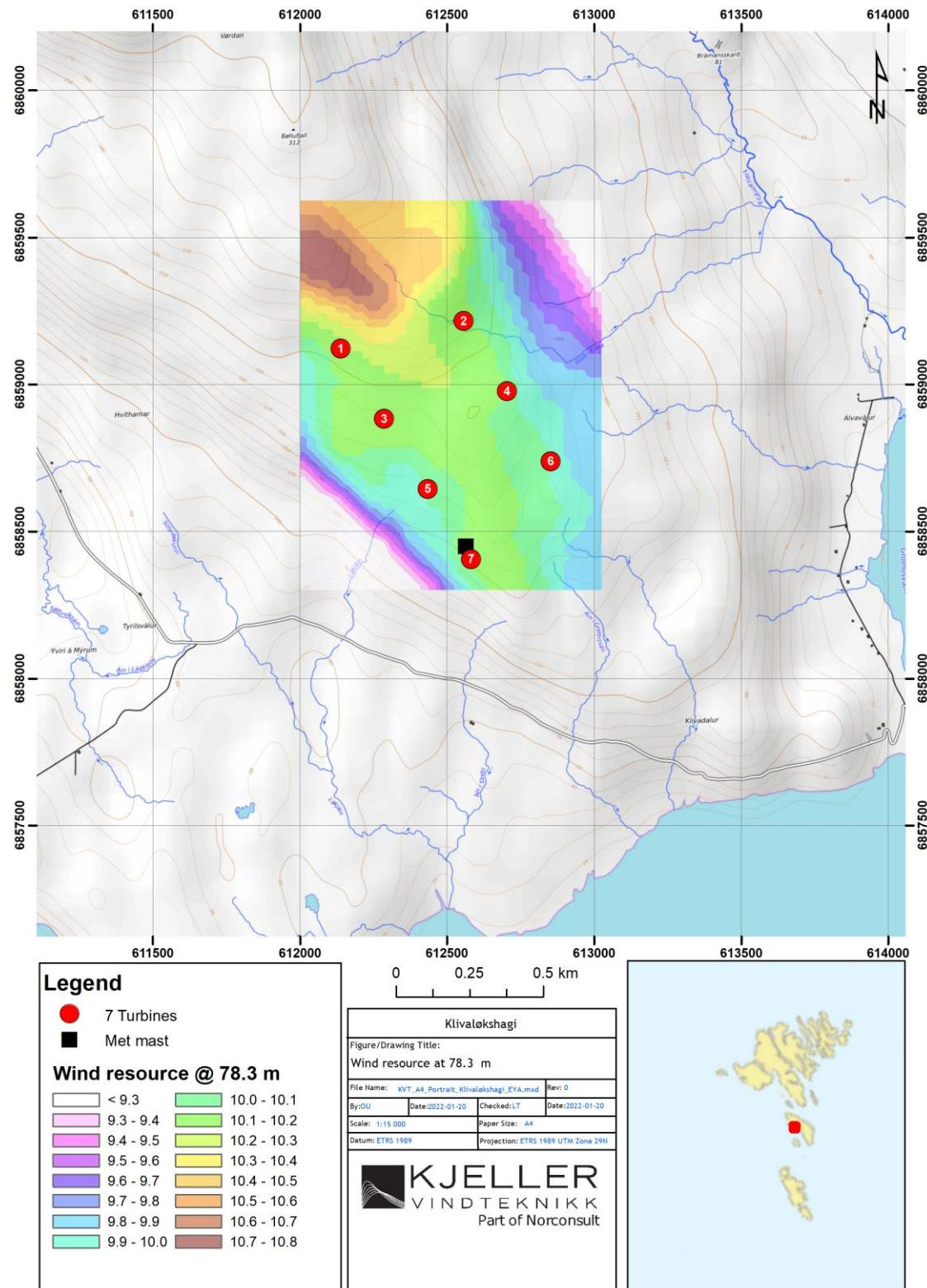
Figure 6. Wind resource map valid at 78.3 m AGL at Klivaløkshagi (together with 7 turbine layout).
