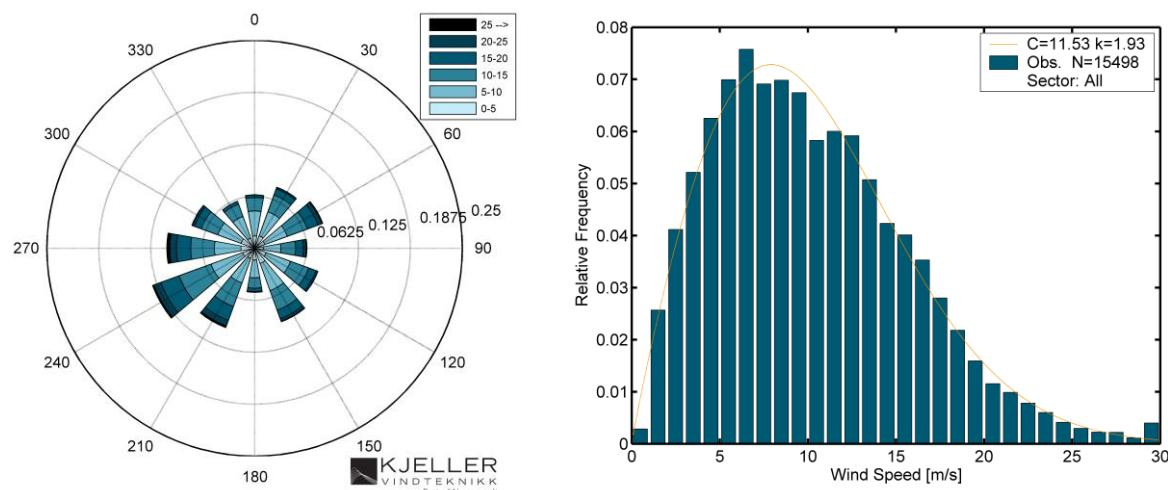
Figure 1. Long term wind rose and Weibull distribution at the site (85.1 m AGL) with KVT Meso as reference data.
