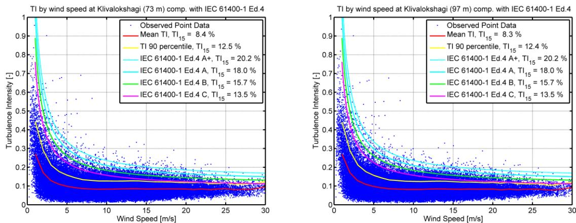
Figure 3. Ambient turbulence intensity as a function of the wind speed.
