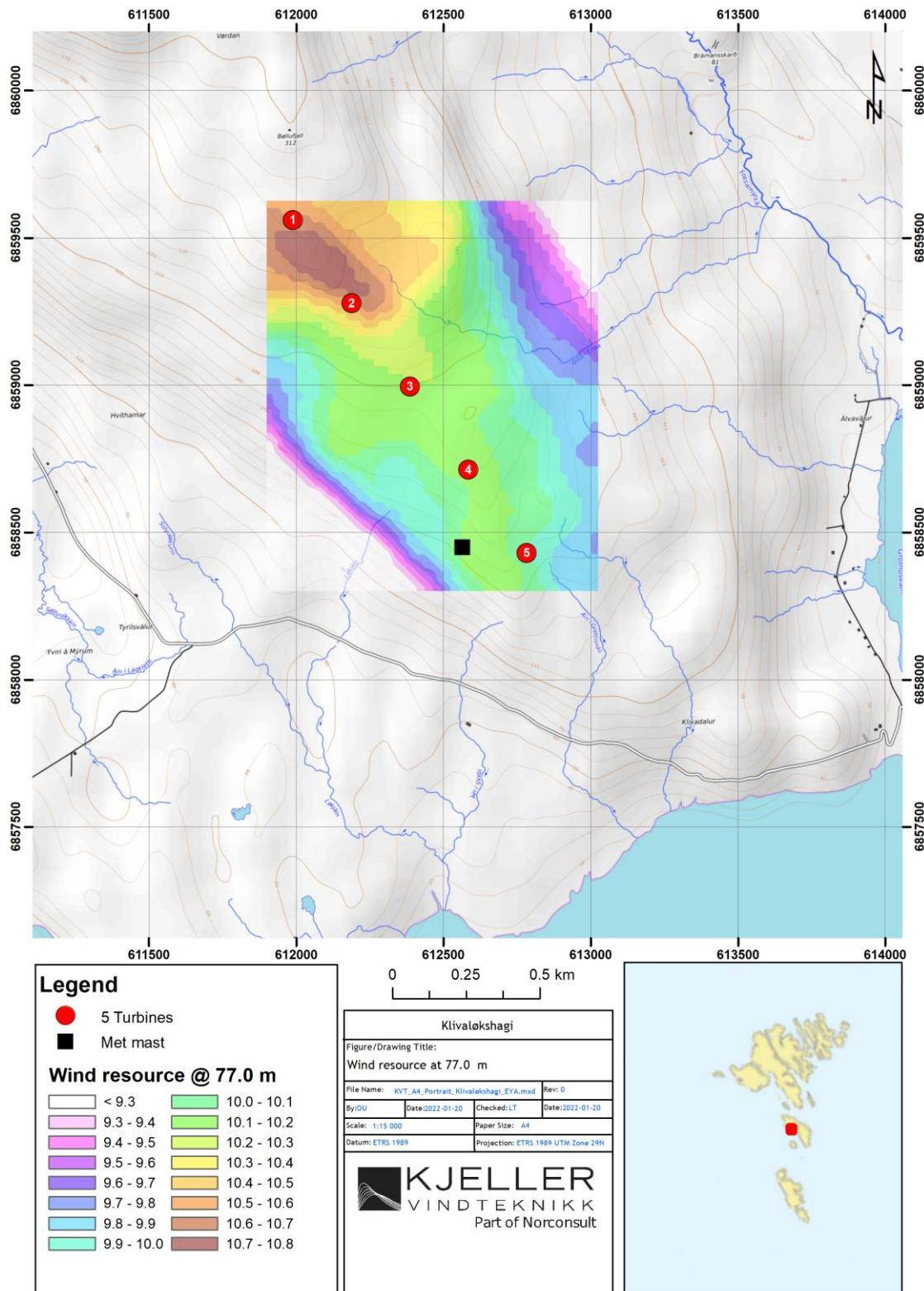
Figure 5. Wind resource map valid at 77 m AGL at Klivaløkshagi (together with 5 turbine layout).
