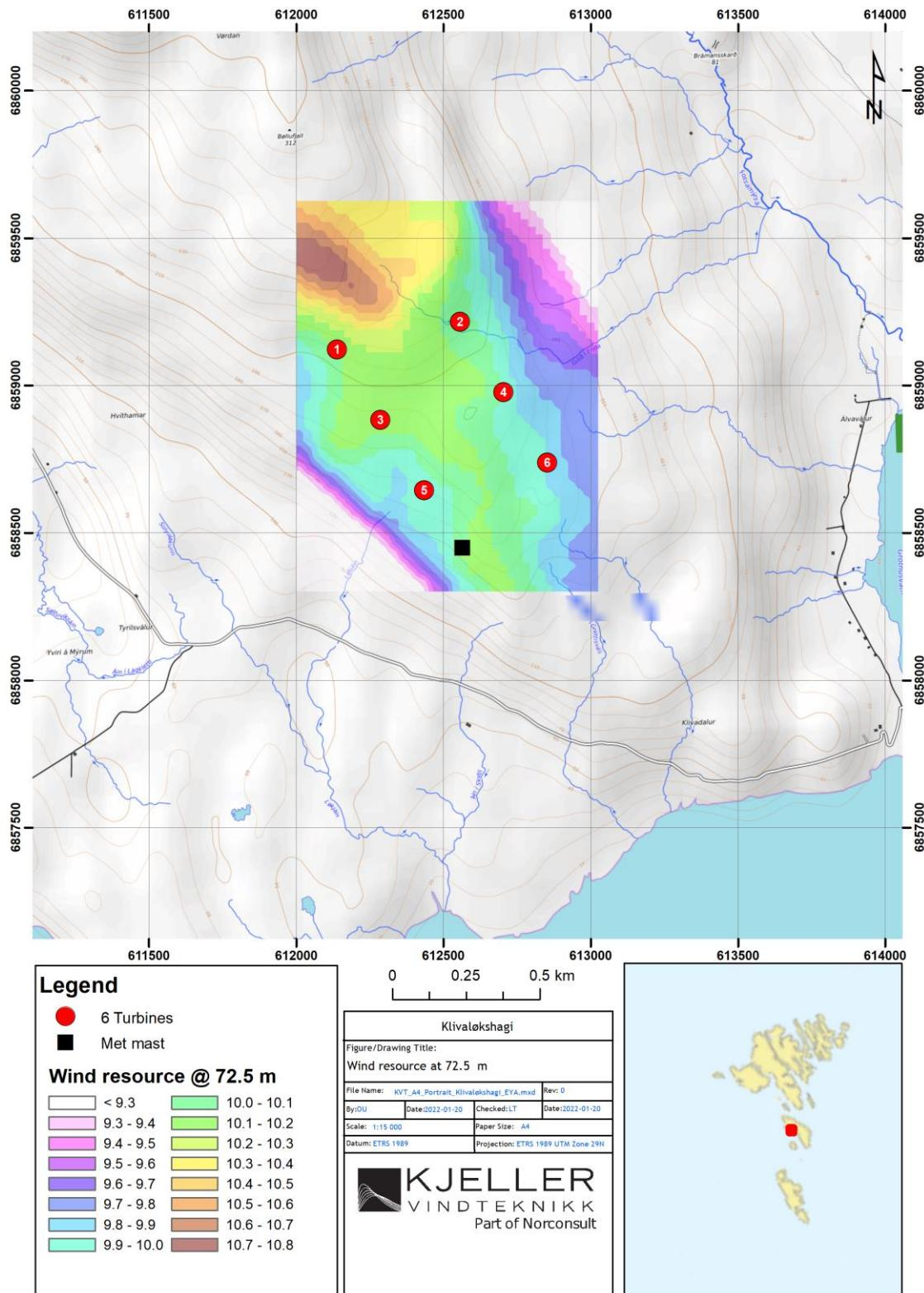
Figure 4. Wind resource map valid at 72.5 m AGL at Klivaløkshagi (together with 6 turbine layout).
