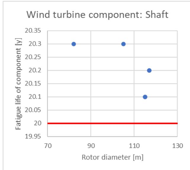
Figure 10. Fatigue life of the shaft as function of rotor diameter (RD) for all IEC IA alternatives.
