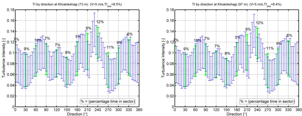
Figure 2. Ambient turbulence intensity as a function of the wind direction. The middle dots mark the mean TI. The upper and lower whiskers mark the mean value plus/minus one standard deviation, respectively. The values presented in the figure show the occurrence frequency of each wind direction sector.
